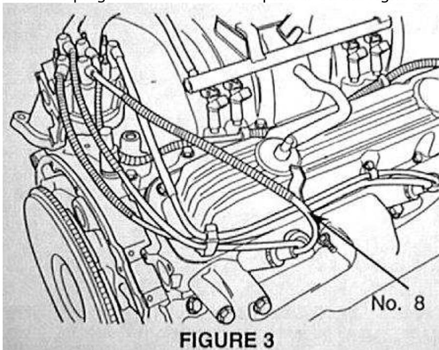
4. Reposition the original piece of plug wire convolute to prevent the wire from chafing at the right valve cover and with other engine components.
