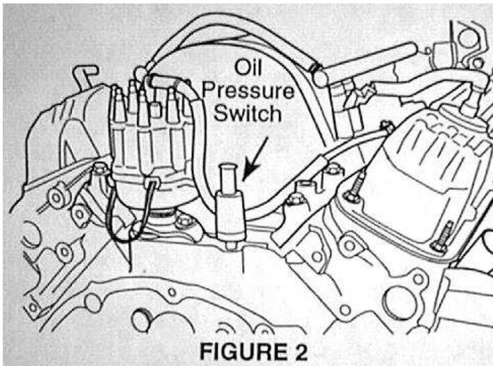
9. Route the distributor end of the coil wire up the side of the distributor cap and onto the coil tower terminal.
