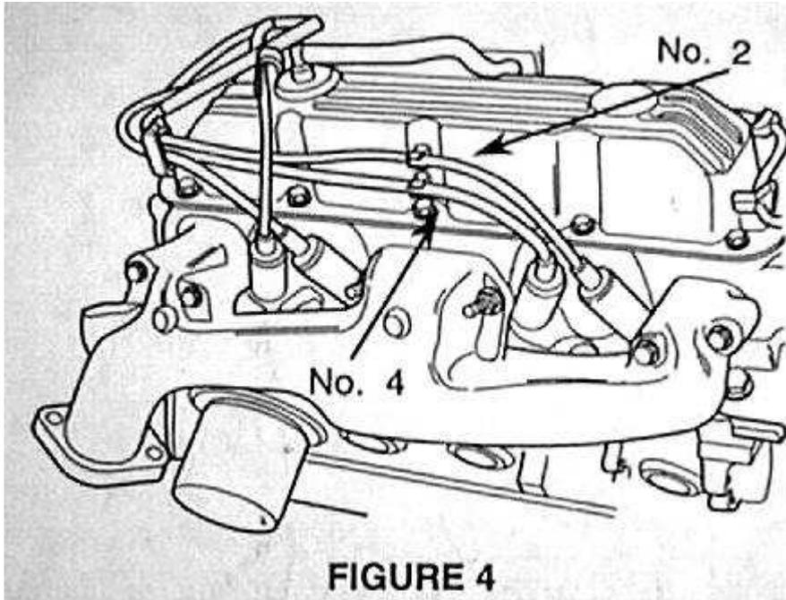
1. Remove the #4 cylinder plug wire from the distributor cap terminal.
